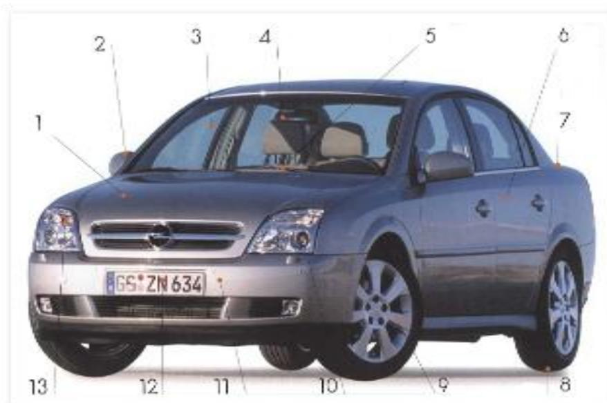
front bumper, front door, front indicator light, driver's seat, rear door, wheel, tyre, rear wing, rear bumper, rear light, trunk, rear window, roof, steering wheel, windscreen, bonnet, front wing, headlight
